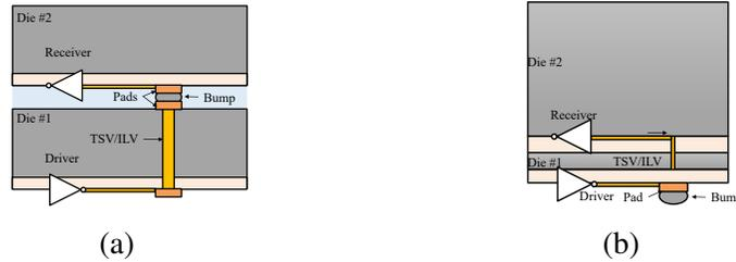
Figure 7.2: Illustration of digital signal channel for (a) TSV and microbump-based and (b) polyolithic and monolithic 3-D integration.
