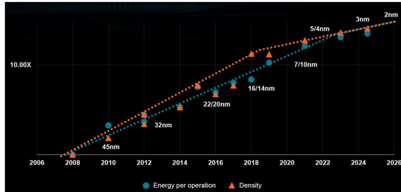
Figure 1.6: Non-linear trend for transistor density and energy per operation. [26]
